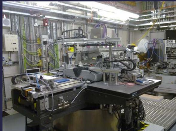
At the back of the hutch there is a newly installed optical table which will provide a more dedicated facility for powder-diffraction studies, including a microfocused beam ( $\sim 10 \mu\text{m}$ ) via a set of KB mirrors housed on a vessel on the table, which will free up the Newport for single-crystal studies. The Newport will also have a less restricted motion.
