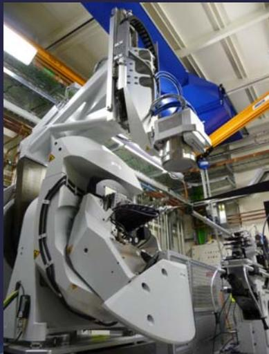
The 4-circle diffractometer was supplied by Newport and has kappa geometry.
