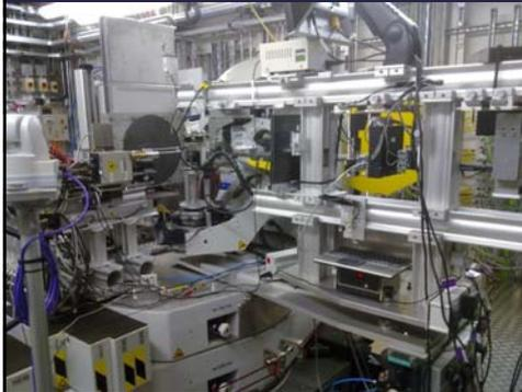
The Newport 6-circle, situated at the front of the experiments hutch, has been used mainly for powder-diffraction studies – the images show it set up in this mode with the MAR 345 image plate detector.
