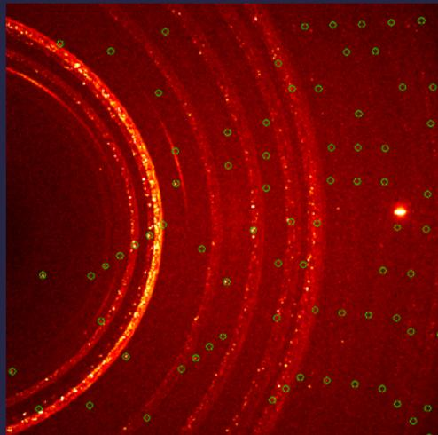
If the incident beam passes through Be then diffraction pattern is contaminated with Be powder pattern:
