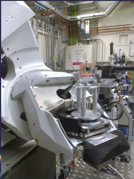
We have been collaborating with Dr Craig Bull of The University of Edinburgh to implement a high-temperature stage for the EH2 diffractometer. This will be fully tested within the next few weeks and we expect to achieve temperatures in the order of 300°C initially.
