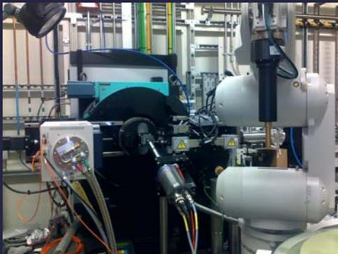
The diffractometer and robotic sample changer were supplied by Rigaku (Saturn 724+ CCD detector).
