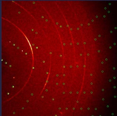
If the incident beam passes through the optical ports in the cell, the Be is not illuminated and the diffraction pattern is relatively clean.
