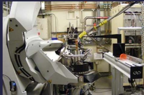
The sample stage, within the phi axis, contains an x,y,z-stage which is capable of carrying 20 kg (repeatability  $< \pm 2\mu\text{m}$ ).
