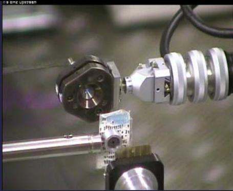
As the diffractometer has a motorised x,y,z-stage within the phi axis it is possible to use scanning techniques to accurately centre the sample (as we'll see in a moment).
