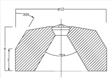
Membrane driven LeToullec type diamond anvil cell, modified for Boehler-Almax anvils.
